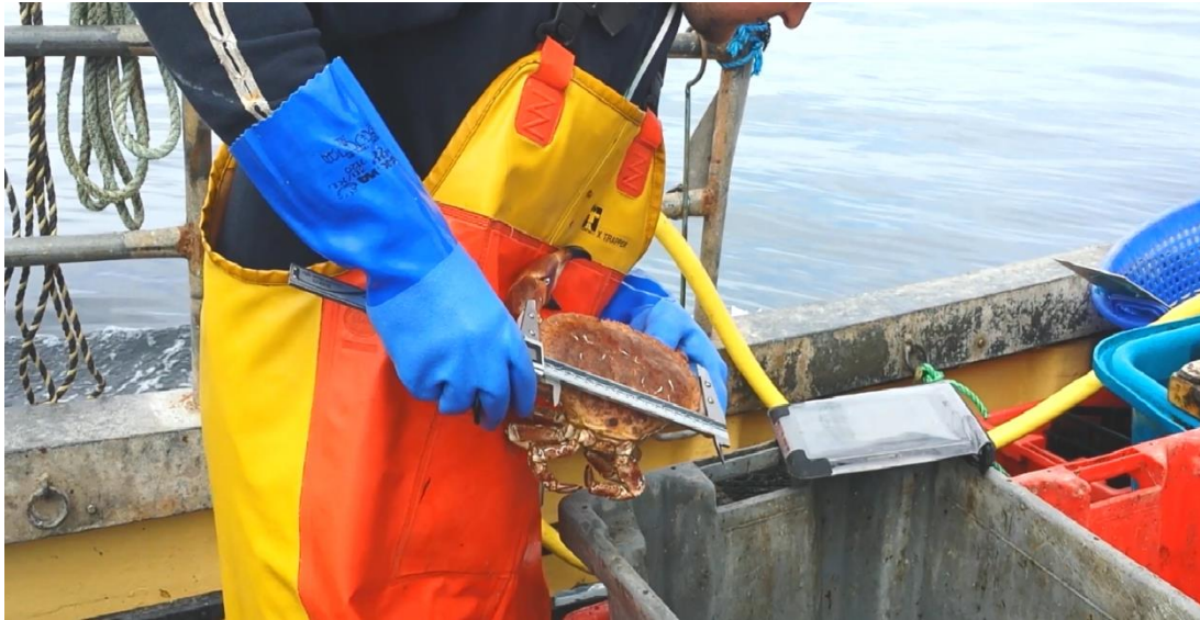
Figure 3. A fisherman using the Bluetooth callipers linked to a tablet, to self-record length data.
